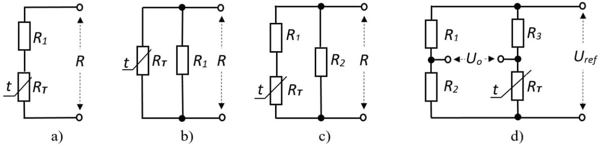
Fig. 2. Correction of the  $R(T)$  thermistor dependence by sequential (a), parallel (b), series-parallel (c) resistor connections and using the non-linearity of the voltage divider in the Wheatstone bridge circuit (d)
